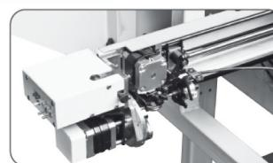
E—Automatically change the spindle sleeve
